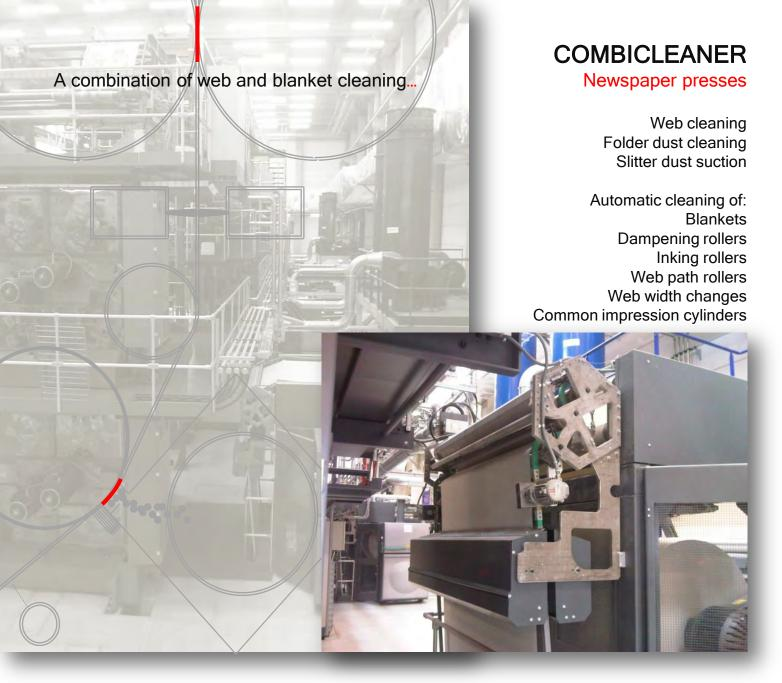
The COMBICLEANER cleaning concept is a combination of techniweb's PAPERCLEANER and TECHNOCLEANER in one complete system.
